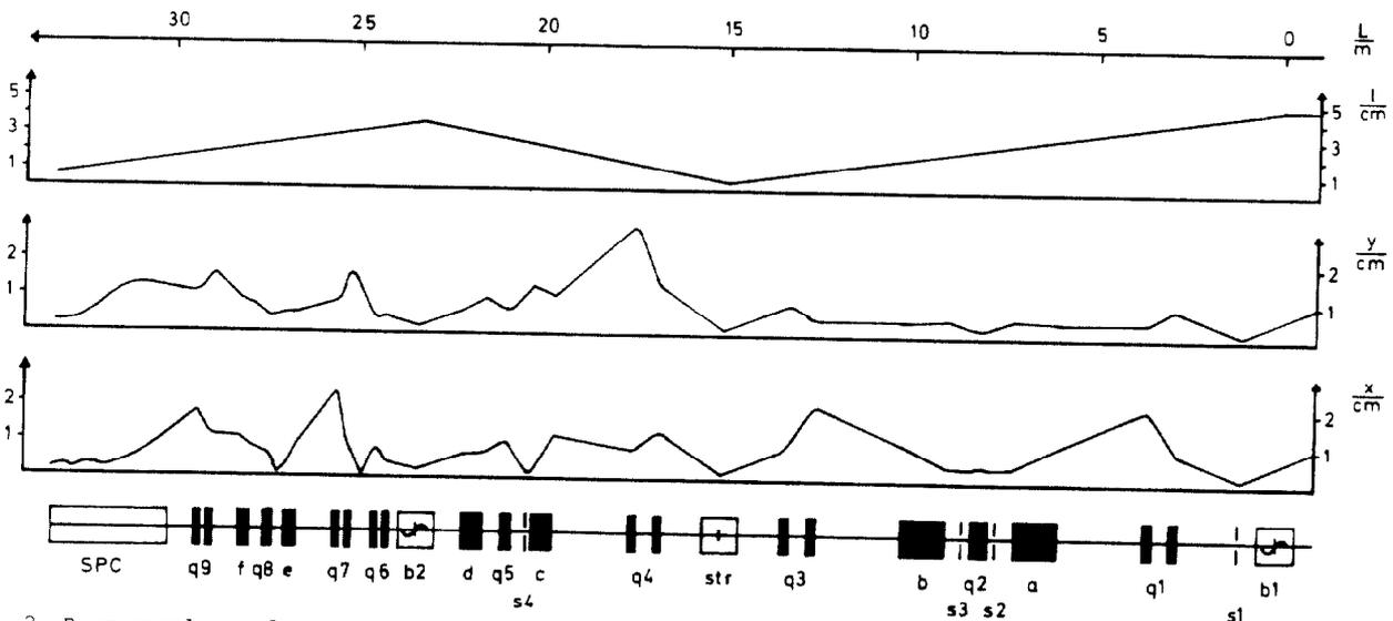
Fig. 2: Beam envelopes for the matching system between the two accelerators in the longitudinal, vertical, and horizontal direction. (Note that the beam moves from right to left.)
