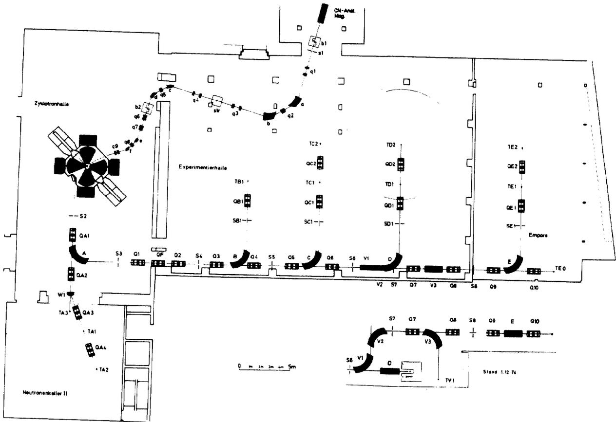
Fig. 1: Layout of the heavy ion accelerator combination VICKSI
