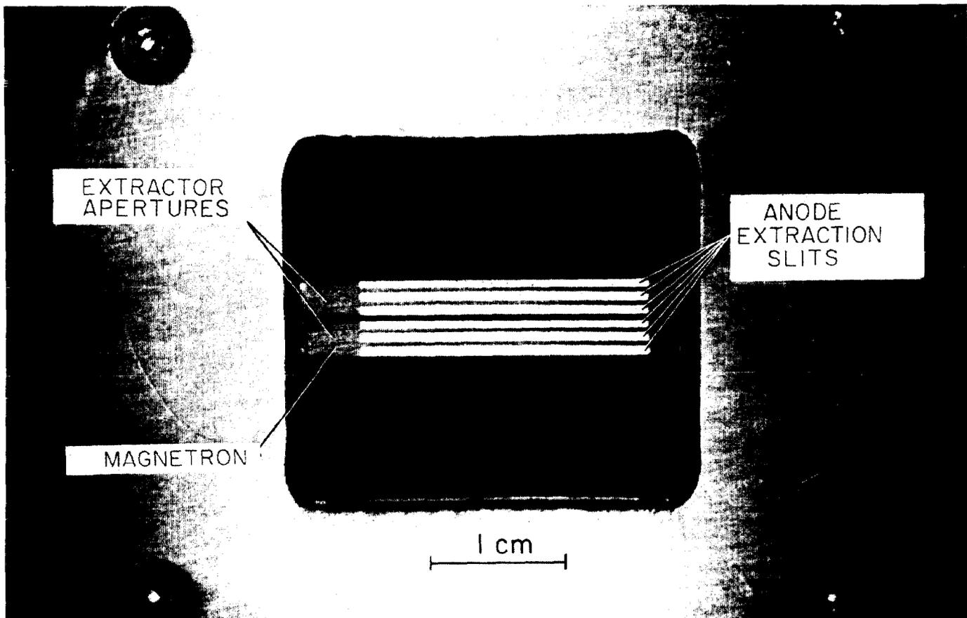
Fig. 5. Close-up of a 120 A discharge in the six slit magnetron.
