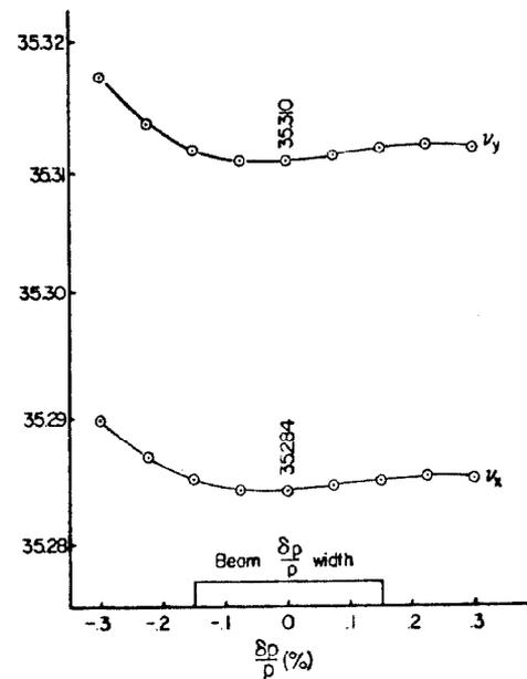
Fig. 2. Vertical and horizontal tunes versus momentum for storage ring lattice after introduction of 160 chromaticity compensating sextupoles in 40 normal cells in each of the north and south arcs.
