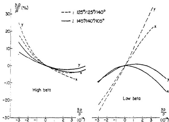
Fig. 3. Fractional change in the amplitude function as a function of momentum at the crossing point in the high angular resolution insertion and in one of the high luminosity insertions, for two settings of the phase adjusting insertions. The numbers separated by slashes at the top of the Figure are the settings of the three phase adjusting insertions in clockwise order starting from the north end of the rings.
