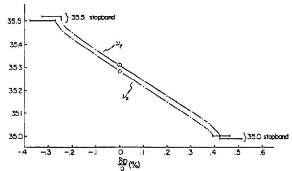
Fig. 1. Vertical ( $\nu_y$ ) and horizontal ( $\nu_x$ ) tunes versus momentum for storage ring lattice before introduction of sextupoles. Stopbands are displaced vertically from one another for clarity.
