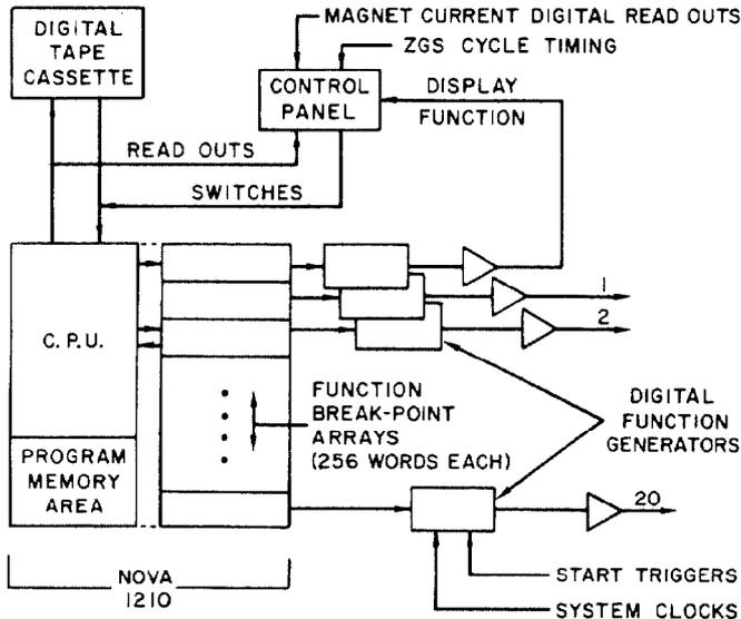
Fig. 4. Functional Block Diagram of Minicomputer-Based Function Generator System
