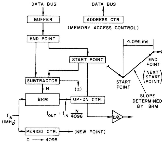
Fig. 5. Digital Function Generator Block Diagram
