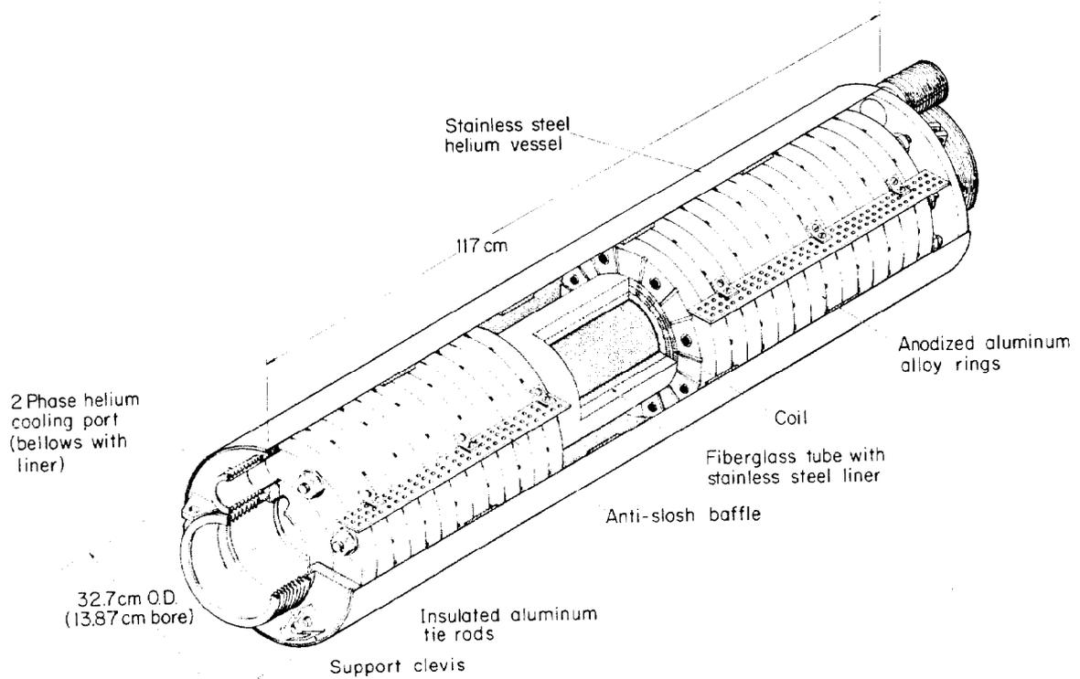
Figure 2 - Dipole-Cryostat Cold Assembly
