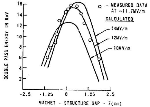
Figure 7: Measured double pass modal energy in MeV vs. magnet to accelerating structure gap.
