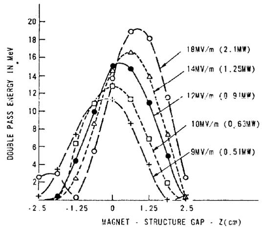
Figure 4: Calculated modal energy in MeV vs. magnet to accelerating structure gap for different field gradients and rf powers (z=0 corresponds to a 1 m drift through the reflecting magnet and back to the structure).
