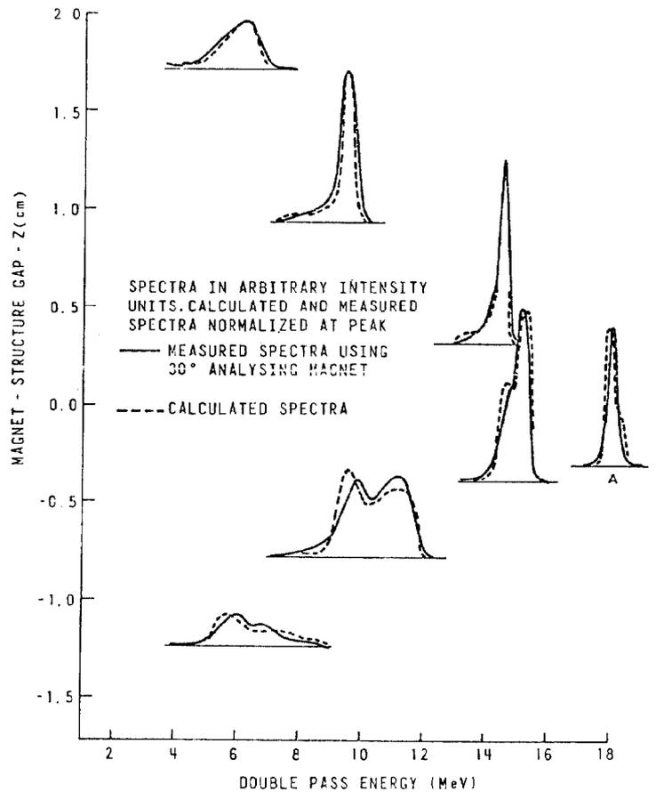
Figure 8: Comparison of measured and calculated energy spectra vs. magnet to accelerating structure gap for a gradient of  $\sim 12$  MV/m (Spectra A at  $\sim 16$  MV/m).
