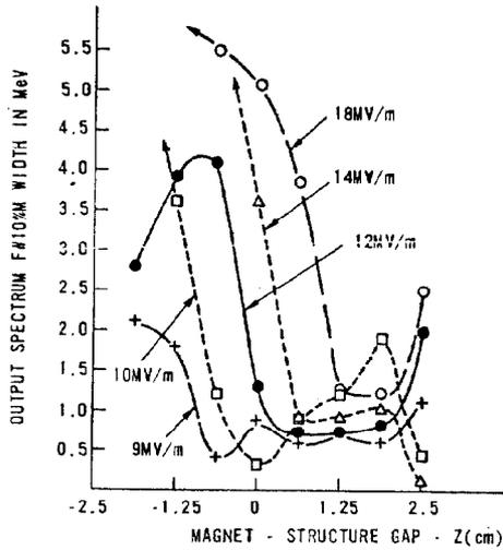
Figure 5: Calculated full spectral width at 10% of the maximum peak height (in MeV) of the double pass energy spectra vs. magnet to accelerating structure gap for different field gradients.
