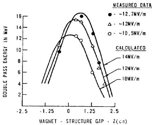
Figure 6: Measured double pass modal energy in MeV vs. magnet to accelerating structure gap for different field gradients.
