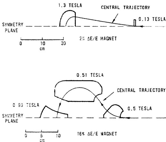
Figure 3: Layout of the two magnet systems (scales approximate). Magnetic fields in Tesla are given for 8 MeV first pass energy.
