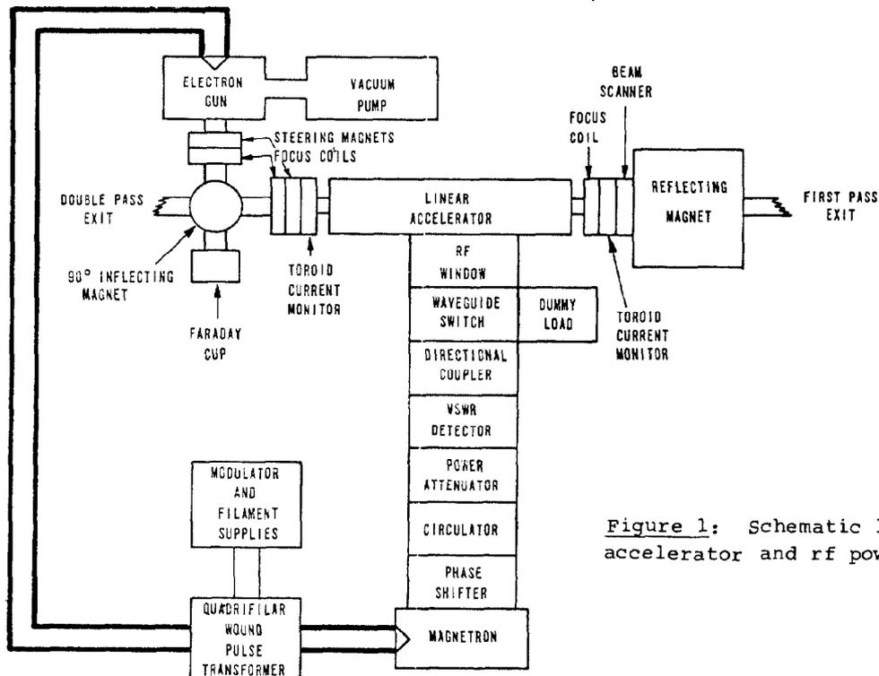
Figure 1: Schematic layout of accelerator and rf power system.
