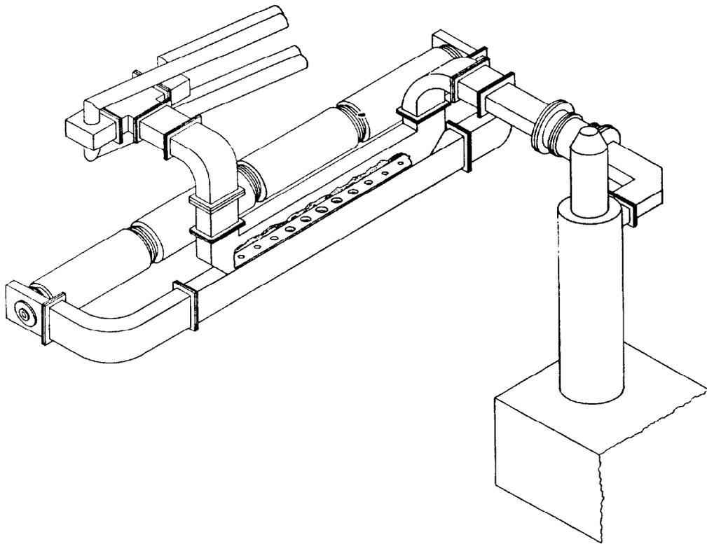
Fig.3. Isometric schematic of the high gradient re-circulating accelerating system.
