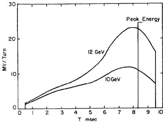
Fig.1. Total voltage per turn versus time required for acceleration to 10 GeV and 12 GeV peak energy.
