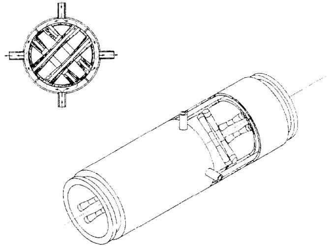
Fig.2. Isometric detail of one cavity section showing water cooling paths.
