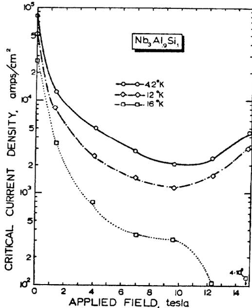
Figure 1 J<sub>c</sub> vs. H for Nb<sub>3</sub>(Al<sub>0.9</sub>Si<sub>0.1</sub>) ribbon; H transverse to J, parallel to plane of ribbon; at 4.2°, 12° and 16°, in He gas.
