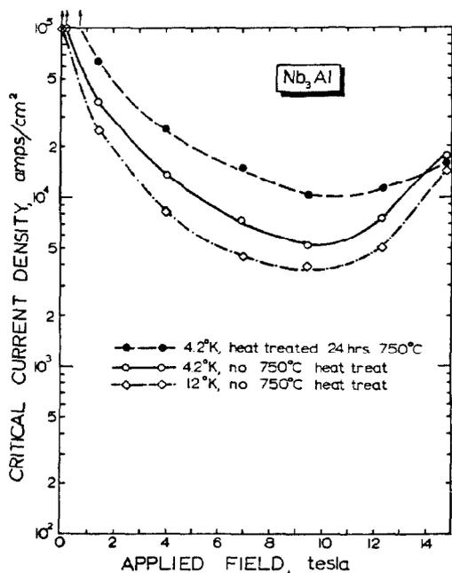
Figure 4 J<sub>c</sub> vs. H for Nb<sub>3</sub>Al ribbon; H as in Figures 1 and 2; at 4.2°K and 12°K for ribbon without 750°C ordering anneal, and 4.2°K with 24 hour anneal at 750°C.
