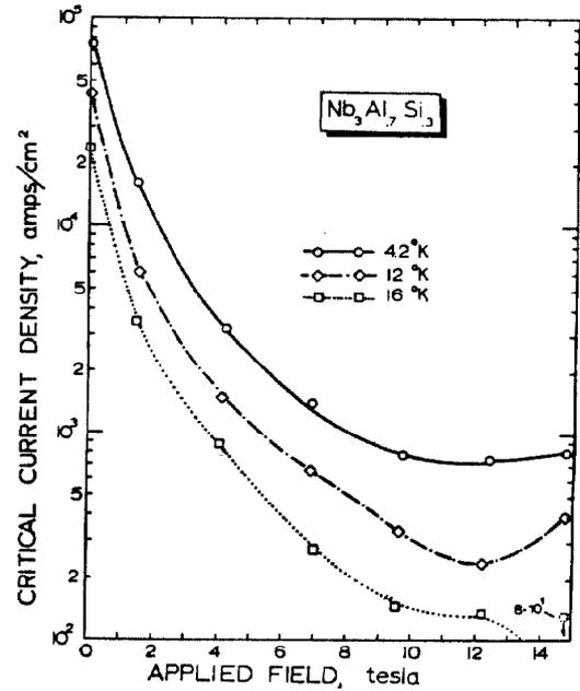
Figure 2 J<sub>c</sub> vs. H for Nb<sub>3</sub>(Al<sub>0.7</sub>Si<sub>0.3</sub>) ribbon; H transverse to J, parallel to plane of ribbon; at 4.2°, 12° and 16°, in He gas.
