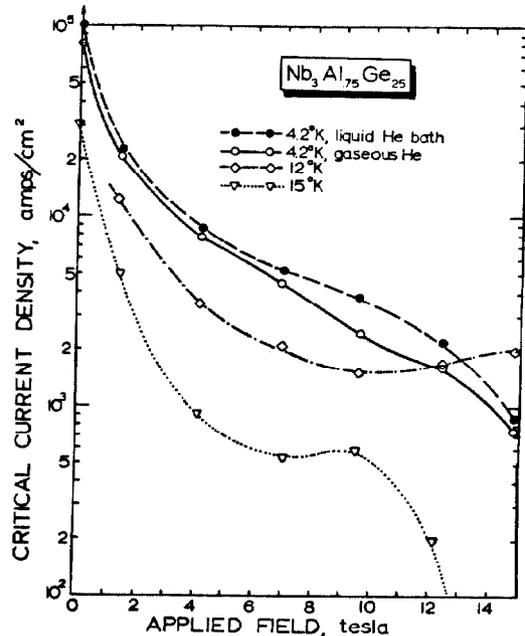
Figure 3 J<sub>c</sub> vs. H for Nb<sub>3</sub>Al<sub>0.75</sub>Ge<sub>0.25</sub> ribbon; H as in Figs. 1 and 2; at 4.2°, 12° and 15° in He gas and 4.2° in He liquid. Note that the liquid environment increases J<sub>c</sub> by ca. 30%.
