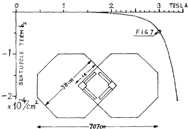
FIG. 6: SEXTUPOLE FIELD TERM OF HIGH FIELD MAGNET
