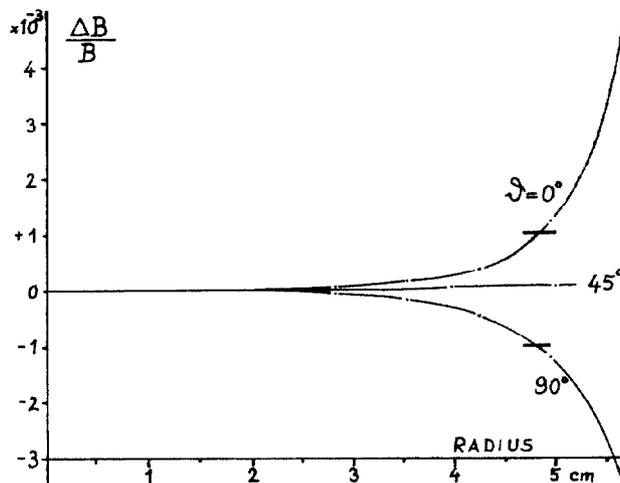
FIG. 4: FIELD HOMOGENEITY OF MAGNET IN FIG. 3
