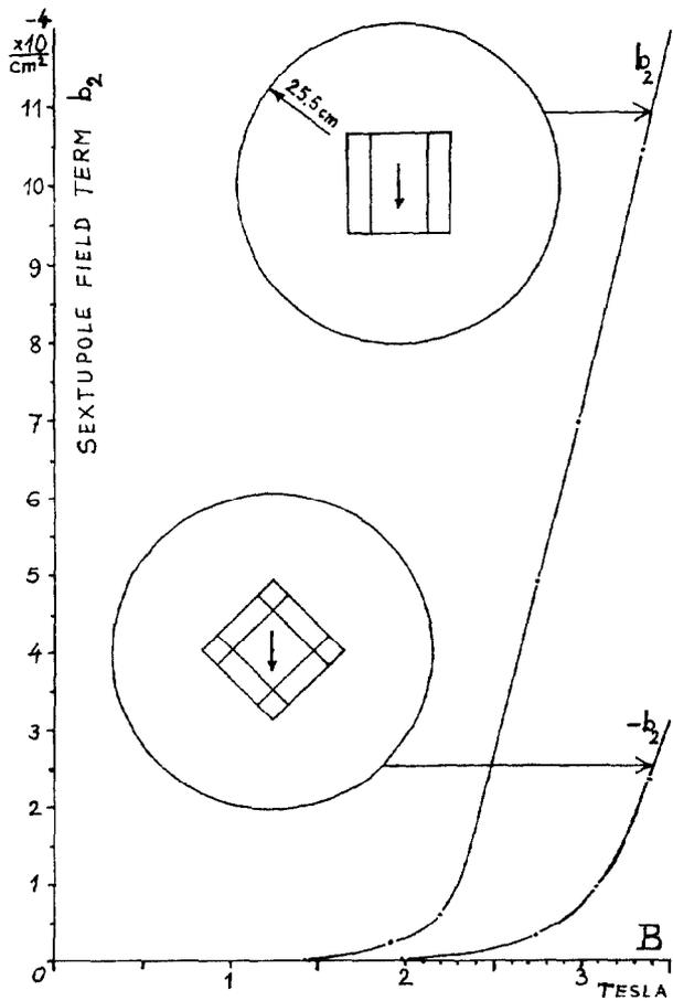
FIG. 5: COMPARISON OF WINDOW FRAME WITH HIGH FIELD MAGNET
