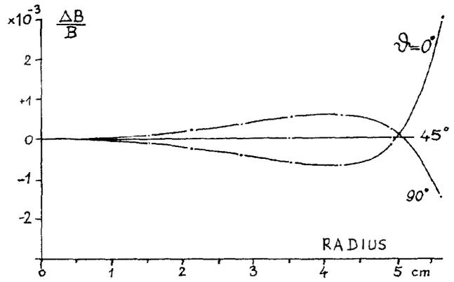
FIG. 7: FIELD HOMOGENEITY AT 30.1 KGAUSS
