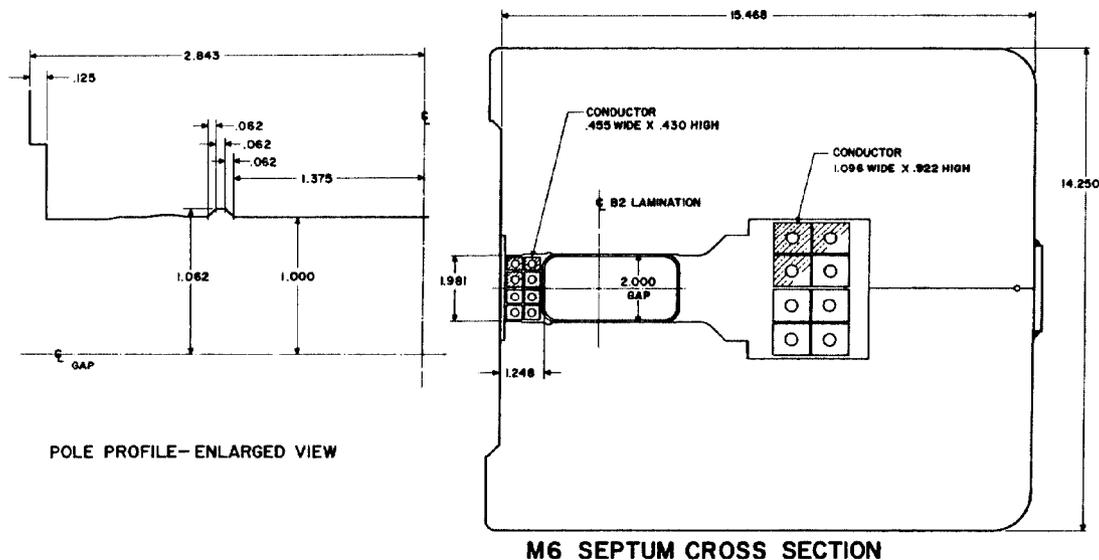
Figure 1. The first of this type is 80.9 ft from the target at its front end and is the first element in the beam line. At that point the separation of the M6 beam from the M2 beam line is 1.47 inches. The notch shown was added to the B2 lamination pole profile in order to improve field quality, based on LINDA Runs. In fabrication it was
