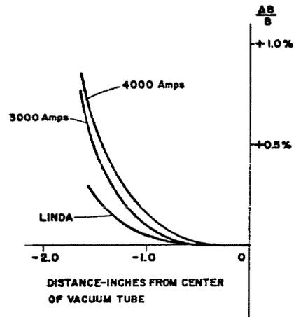
Figure 4. Shown here are two measured curves and a curve from the LINDA calculation of the M1 magnet. The different behaviour at the two currents is due to saturation effects at the higher current.
