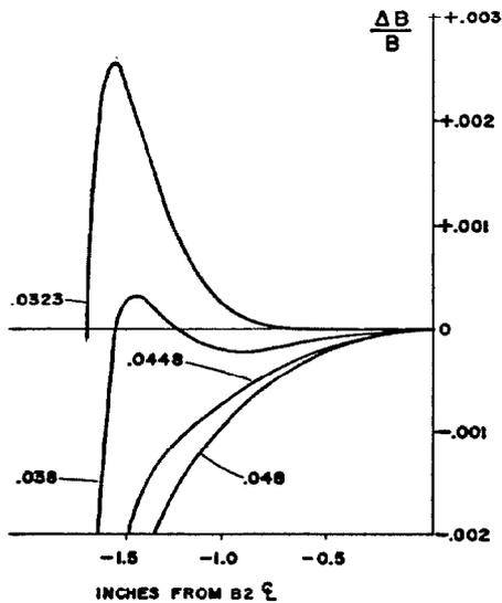
Figure 5. These curves illustrate the variation of the  $\Delta B/B$  behaviour with changes in the size of the shim between the upper and lower halves of the septum coil. The label is the half-size of the shim in inches.
