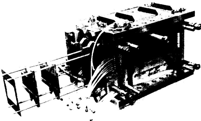
Fig.4  $\Lambda$  Dipole Assembly partly dismantled to show restraining members, and with Polaroid film plate telescope fitted.
