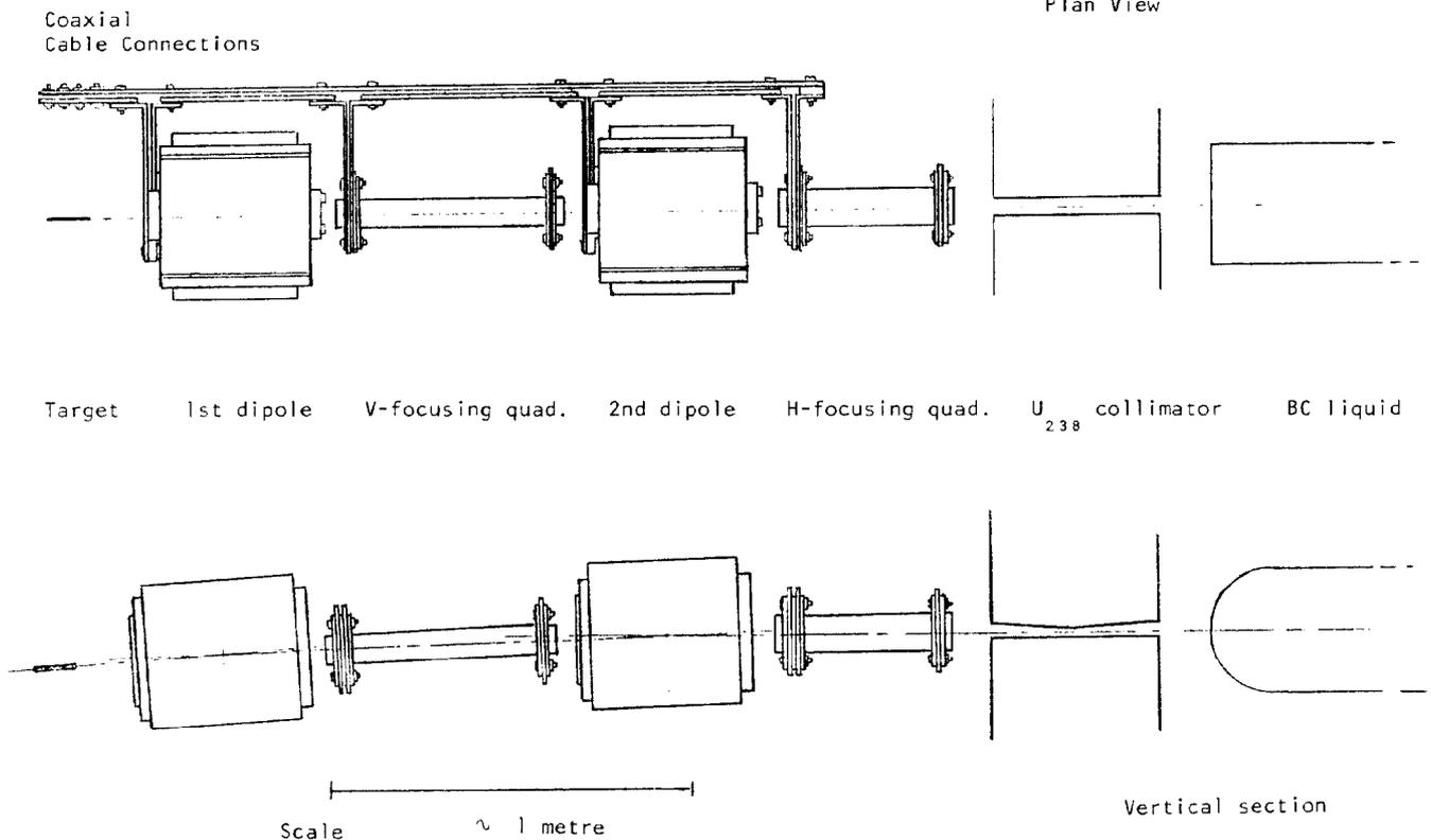
Fig. 1 General layout of a Pulsed Beamline as envisaged for a 20 GeV/c  $\Sigma^-$  Experiment at CERN
