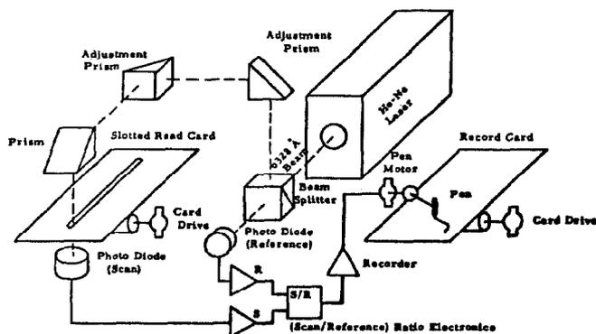
Figure 2. Schematic of the TFD Reader
