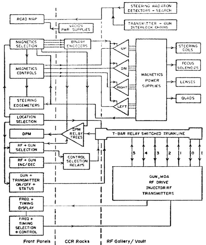
Fig. 3 - Block Diagram of Gun, Transmitter and Magnetics Controls and Metering in CCR
