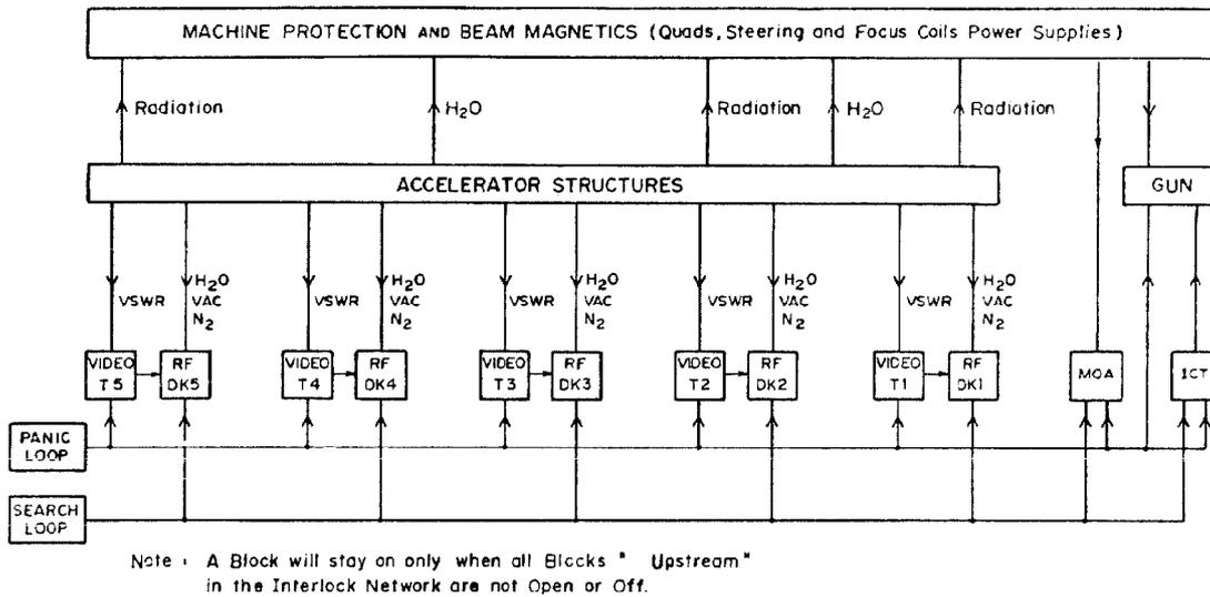
Fig. 5 - Main Accelerator Interlock Loops
