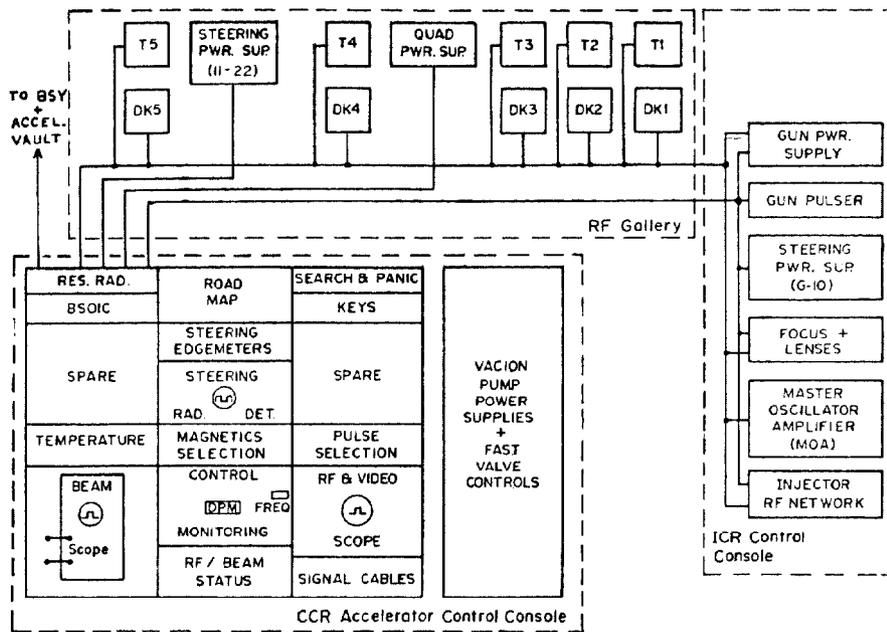
Fig. 4 - Block Diagram of Accelerator Controls
