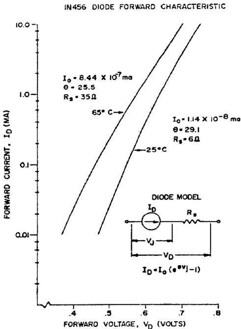
Figure 3. Forward I-V Characteristic For 1N456 Diodes with Diode Model and Fitting Functions Specified.
