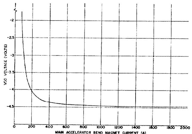
Figure 1. Radio Frequency Voltage-Controlled Oscillator Drive Required as a Function of Main Accelerator Bend Magnet Current.
