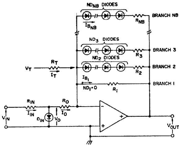
Figure 2. Basic Non-Linear Transfer Function Generator Utilizing Forward Biased Diodes.
