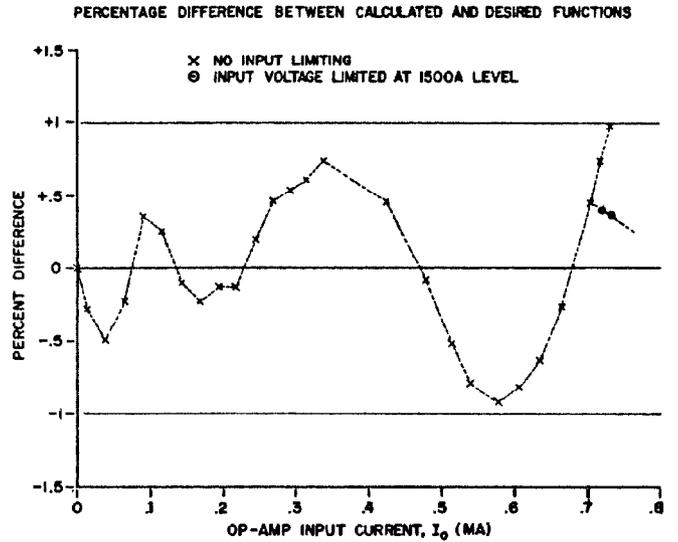
Figure 4. Percentage Difference Between the Circuit Performance and the Desired VCO Drive Voltage After Convergence.
