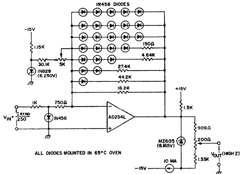
Figure 5. Function Generator to Provide Radio Frequency VCO Drive as a Function of Main Accelerator Bend Magnet Current.
