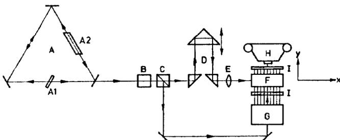
Fig.2 Experimental set-up. A laser resonator, A1 saturable dye, A2 laser rod, B KDP-crystal, C beam split for dividing green and IR-pulses, D delay, E focusing lens, F Kerr cell filled with  $\text{CS}_2$ , G beam expander, H camera, I crossed polarizers.
