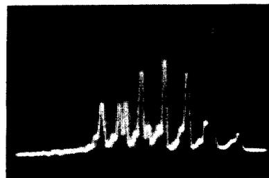
Fig.7: Oscilloscope-trace of a sampled bunch. Time 50 nsec/div. The scope picture was photographed by means of an image converter tube.
