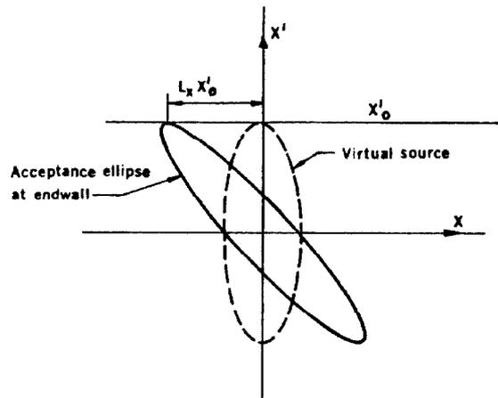
Fig. 3. Relationship of beam ellipse at poststripper end wall and virtual source.
