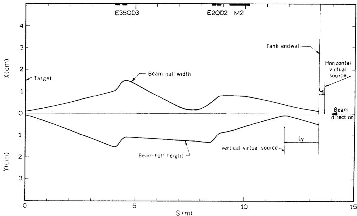
Fig. 5. Beam envelope and virtual source positions for line E35.
