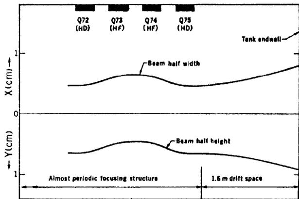
Fig. 2. Beam envelope at poststripper exit, calculated from transverse focusing forces.
