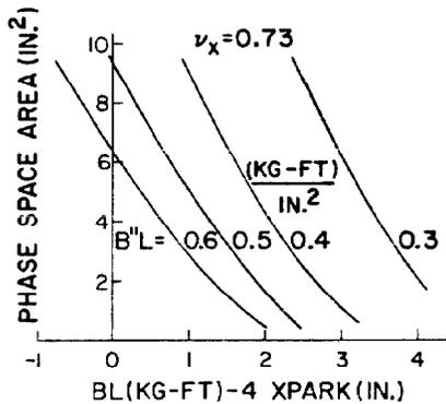
Fig. 3 Stable Phase Space Area as a Function of Sextupole Field, Dipole Field, and Equilibrium Orbit Position
