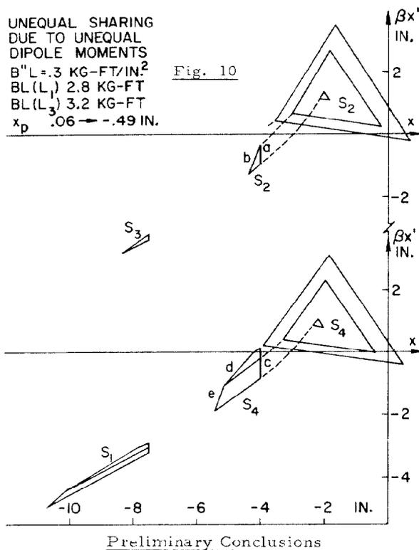
Simultaneous  $\nu_x = 2/3$  resonance extraction into the two ZGS proton areas appears to be feasible and attractive. Slow spills (with rf structure) should be possible using a sum signal from the proton areas to control the rate of spill and a difference signal (applied say to one of the dipole coils in the L1 or L3 magnets) to control the sharing. Slow spills without rf structure will be possible after active ripple suppression on flattop for the ZGS is accomplished (in perhaps six
