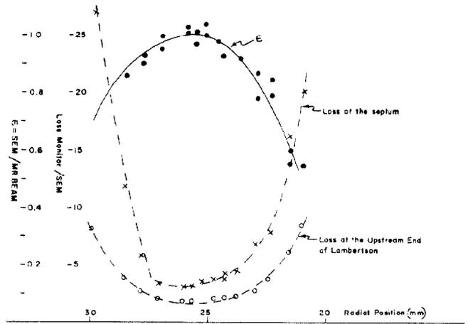
Fig. IV. Extraction efficiency and losses for different radial positions of the septum.
