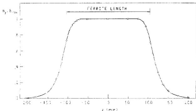
Fig. 1: Normalised flux density of the magnet along the beam axis z.
