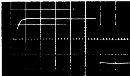
Fig. 3: The current pulse shape; horizontal line scale 20 μs/large division.
