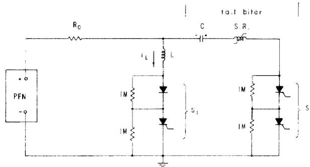
Fig. 2: The pulser circuit.
