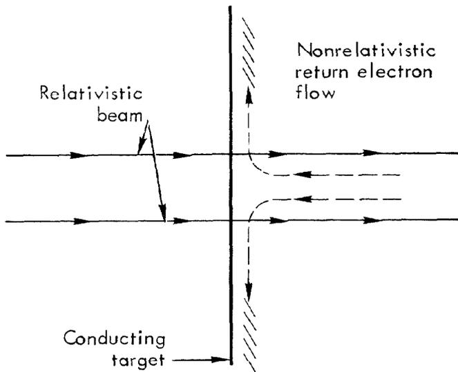
Figure 6. Acceleration of electrons by magnetic compression and axial electric field.
