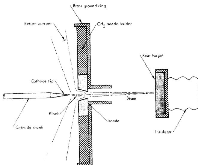
Figure 3. Relativistic pinch gun geometry.
