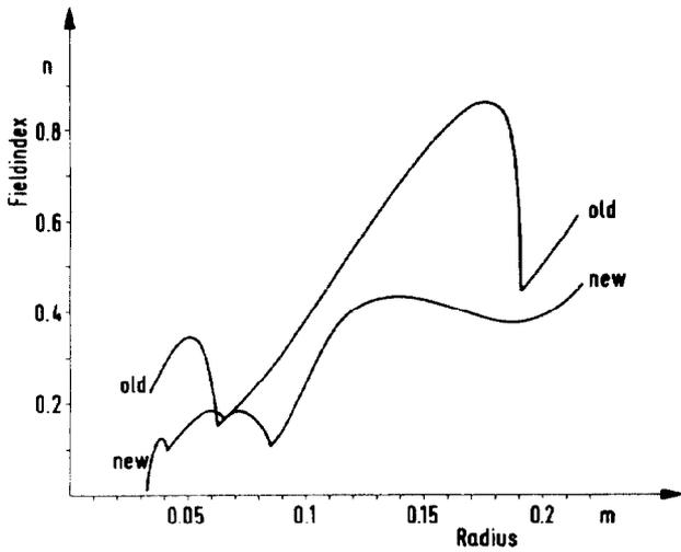
Fig. 3: Fieldindex  $n$  as a function of  $R$  in the old and the new set up
