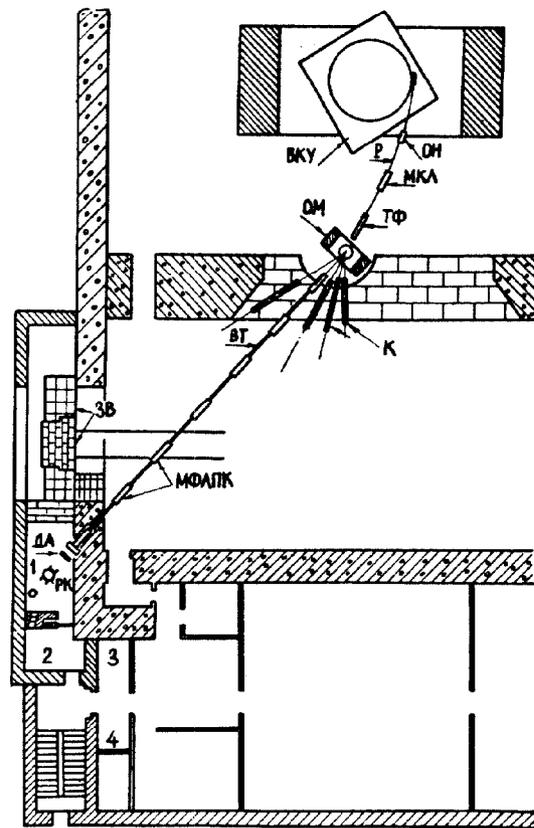
FIG. 3--Proposed variant of beam distribution and the plan of experimental halls after reconstruction the JINR synchrocyclotron. At the bottom of the drawing a vertical section of the system for transportation of the primary proton beam and a scheme of focusing of the therapeutic  $\pi$ -meson beam by wide angle magnetic lens.
