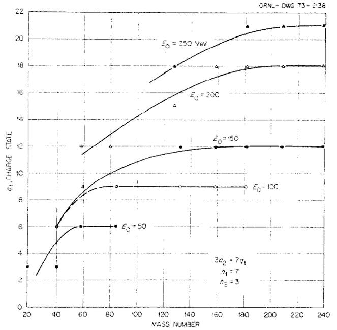
Fig. 5. Ion source charge states required for conditions of Fig. 4. The charge states must be integers. The curves indicate trends, only.
