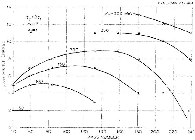
Fig. 3. Ion source charge states required for conditions of Fig. 2. The charge states must be integers. The curves indicate trends, only.
