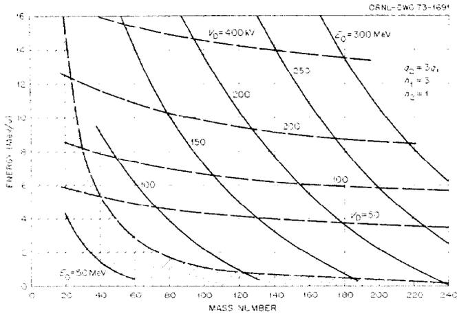
Fig. 2. Energy obtainable for various sizes of cyclotrons with recycling and 3:1 stripping. The shaded area represents the capabilities of an  $E_0 = 100$  cyclotron without recycling.
