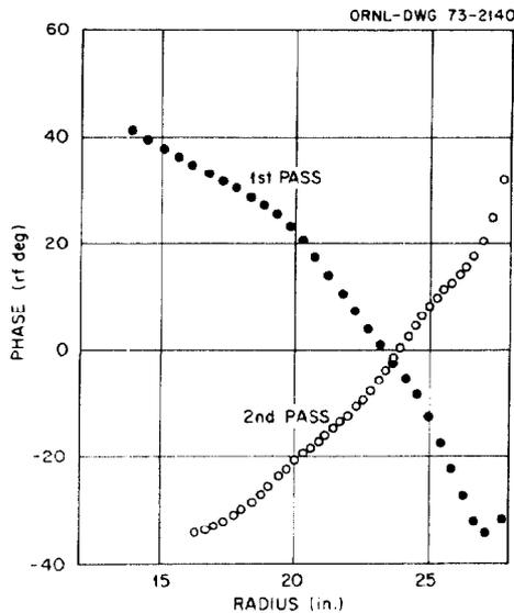
Fig. 8. Phase vs radius for the two trajectories shown in Fig. 7. The opposite, approximately equal phase slips reflect a trim coil adjustment falling between the isochronous settings for the two beams.
