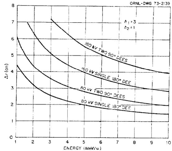
Fig. 6. Turn spacing available for the stripping foil assuming a beam phase of  $40^\circ$  at the foil radius.
