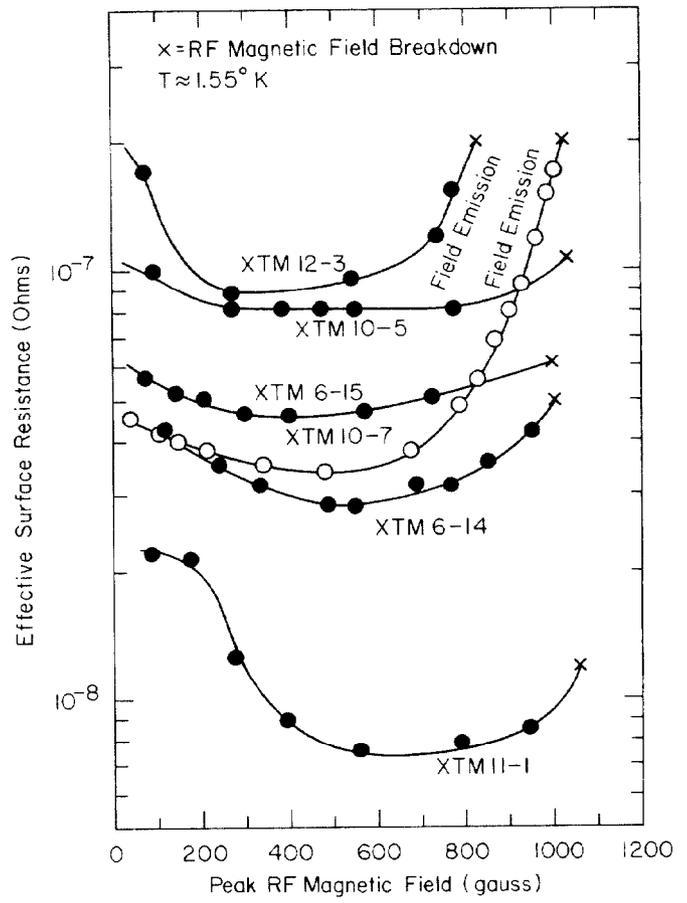
FIG. 2--Effective surface resistance as a function of peak rf magnetic field for several high field cavities.
