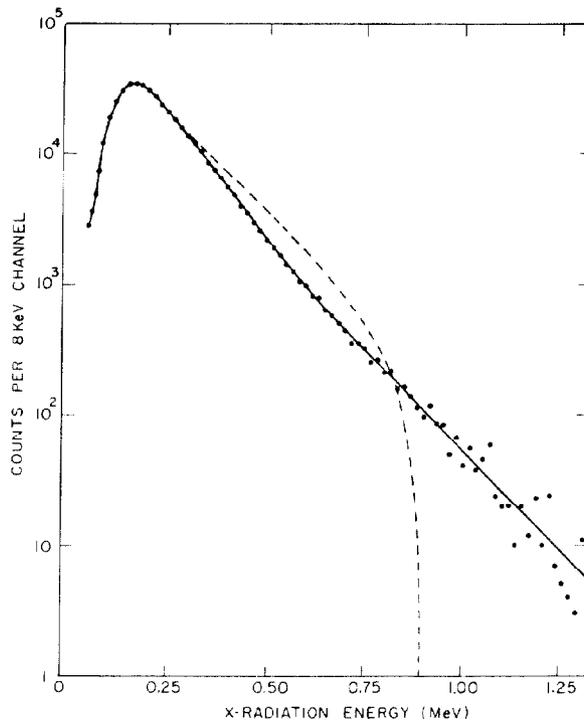
Fig. 2. X-radiation energy spectrum from a superconducting L-band cavity. The dashed line is a calculated x-radiation energy spectrum based on the electron multiplication simulation program.
