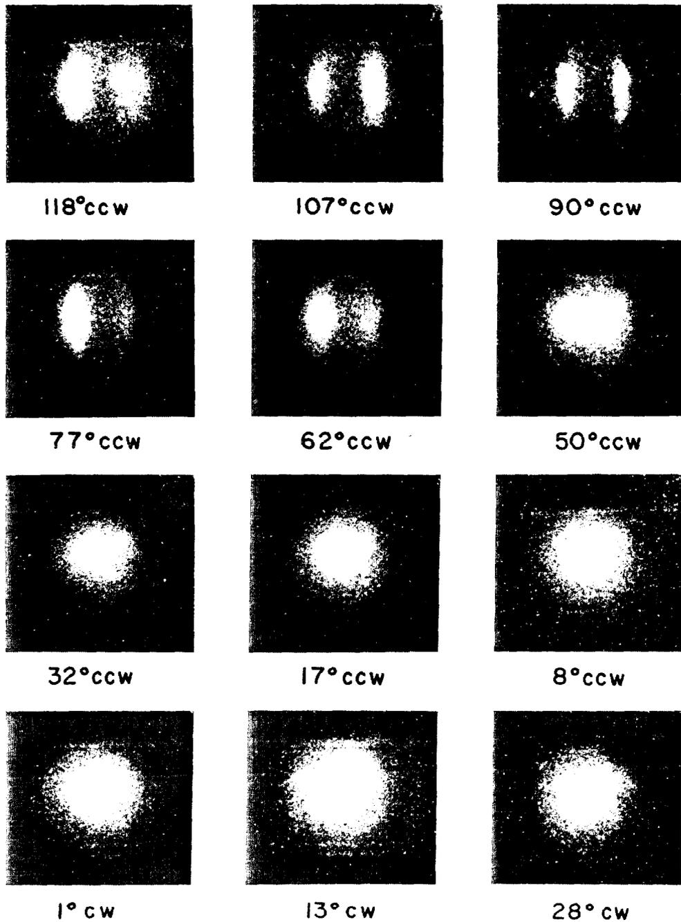
Fig. 1. Series of x-ray photographs from different directions of L-band cavity without beam pipes. The different photographs are for various angles between the cavity axis and the x-ray camera axis.
