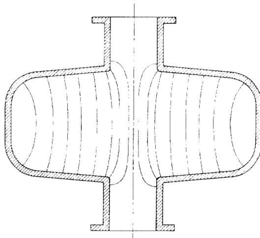
Fig. 1. Cross-sectional view of single-cell L-band cavity with electric field lines indicated by solid lines.
