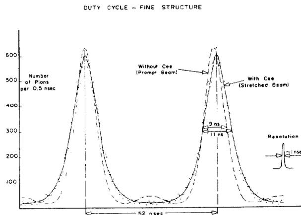
Fig. 2. Fine structure of the beam intensity with and without the Cee.
