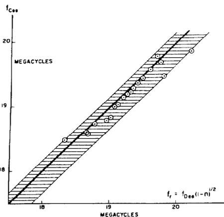
Fig. 3. The Cee frequency at maximum beam intensity versus the frequency of radial oscillation calculated from the Dee cutoff frequency and the magnetic index.
