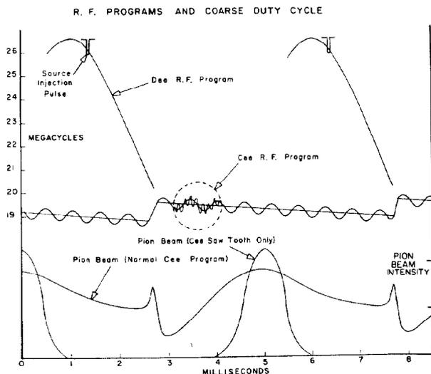
Fig. 1. Dee and Cee r.f. modulation program in the regenerative mode of operation and the coarse duty cycle of the beam intensity.
