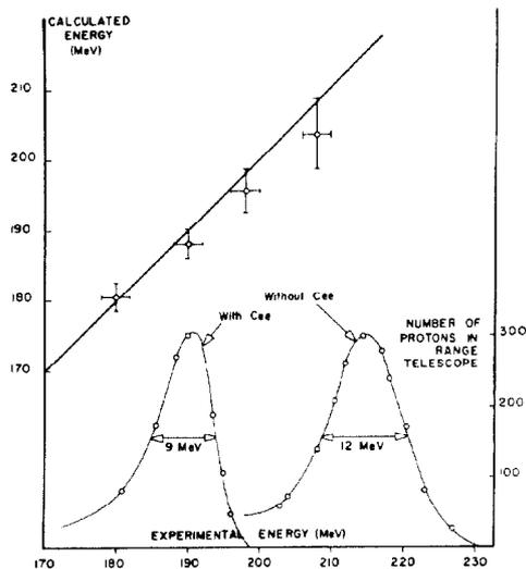
Fig. 4. -TOP- Four proton beam energies calculated from the Dee cutoff frequency, the magnetic field, and the energy loss in the target versus the experimentally measured energies. -BOTTOM- Experimental range curves plotted in terms of energy with and without the Cee.
