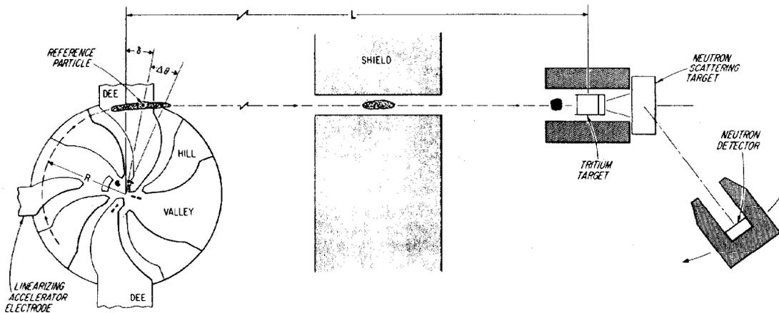
Fig. 2. A schematic view of a neutron time-of-flight scattering experiment.
