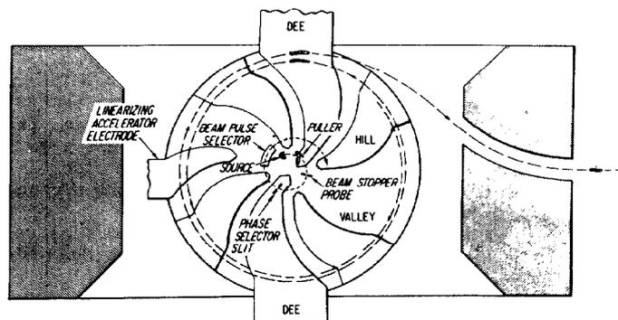
Fig. 1. A schematic view of the NRDL cyclotron showing the special components used for the formation of short beam pulses.
