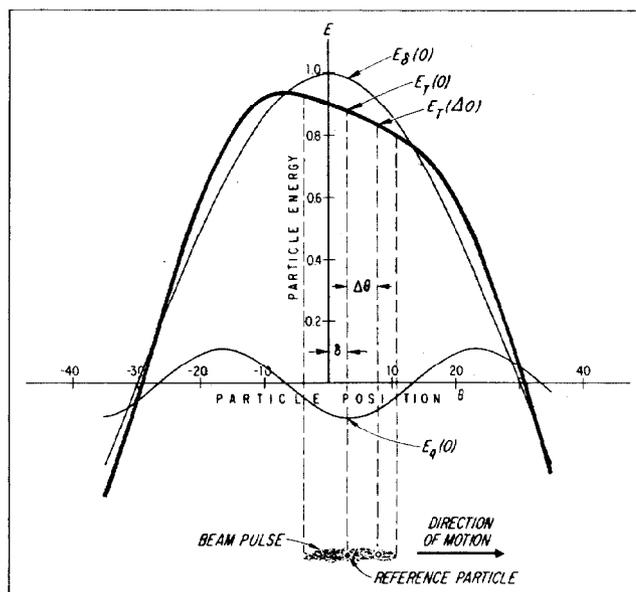
Fig. 3. Linearization of the sinusoidal particle-energy characteristics by the addition of a ninth harmonic.
