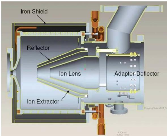
Figure 5: Electron collector for the RHIC EBIS.
