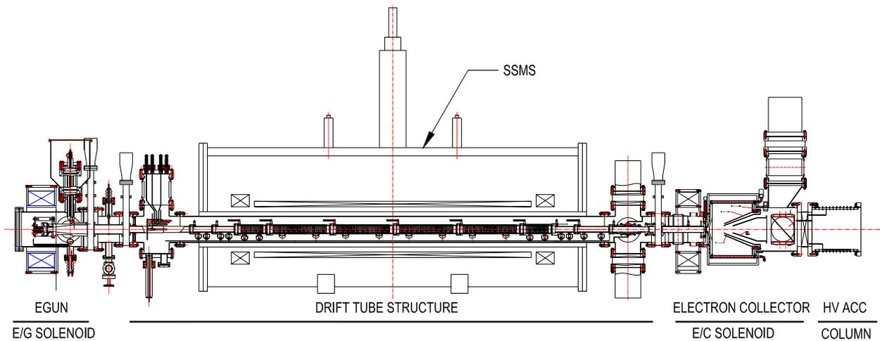
Figure 4: Schematic of the EBIS for RHIC.
