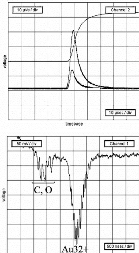
Figure 3: Au ions produced with a 6.8 A electron beam and 36 ms confinement, 4.0 mA peak;  $2.0 \times 10^{11}$  charges/pulse. Charge state distribution peaked around  $\text{Au}^{32+}$
