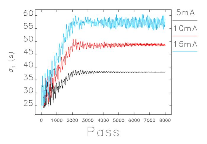
■ The oscillation amplitude is about 2 ps close to the APS streak camera limit.
