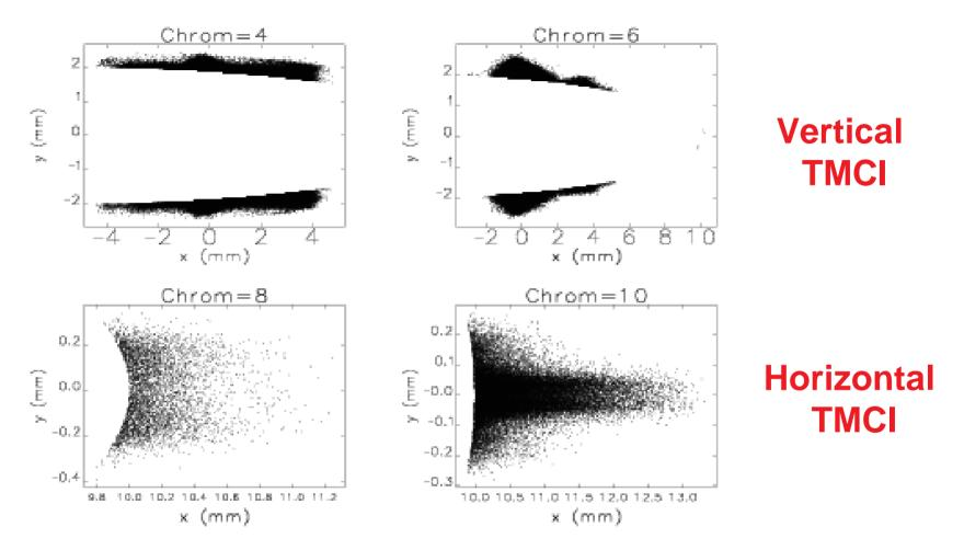
■ Effect of amplitude dependent tune shirt changes beam-loss plane from vertical to horizontal plane.
