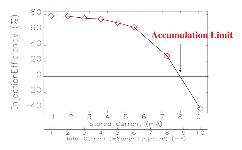
**Measured Accumulation Limit < 8 mA**
