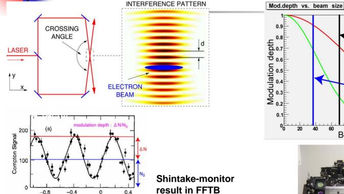
FFTB ~70nm -> ATF2 37nm modification : Laser wavelength fringe stabilization FB
