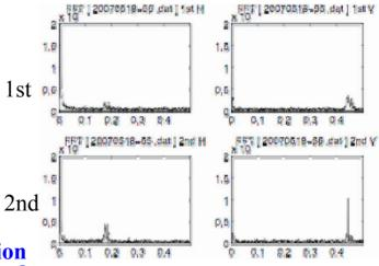
The preliminary results shows the different oscillation amplitude of the tune-X and the tune-Y for the 1st and 2nd bunches at just after injection.
