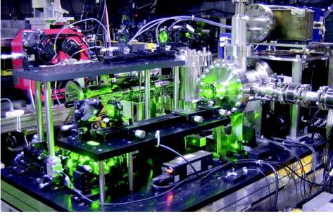
300mW 532nm Solid-state Laser fed into optical cavity
