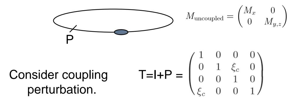
In x-y space,  $\xi_c$  is skew quad strength, In x-z space,  $\xi_c$  is crab cavity strength.
