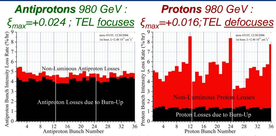
At present, beam-beam effects are relatively stronger on protons, accounting for some 10-15% loss of the integrated luminosity. Proton loss rates vary greatly from bunch to bunch. The Tevatron Electron Lens #2 aligned on **proton** beam.
