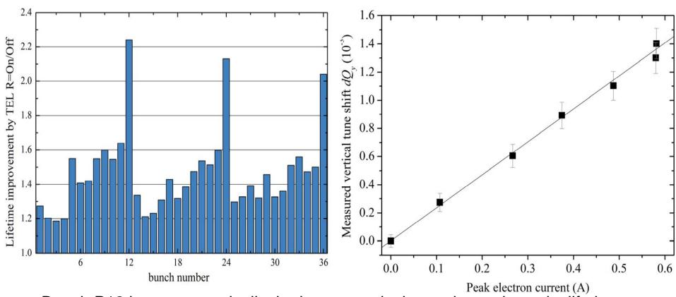
Bunch P12 has systematically the lowest vertical tune that reduces its lifetime (too close to 7/12 resonance). TEL2 raises the tune up by dQ=+1.5e-3
