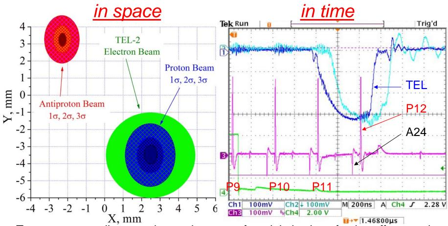
Transverse e-p alignment is very important for minimization of noise effects and optimization of positive effects due to e-beam. Timing is important to keep protons on flat top of e-pulse – to minimize noise and maximize tune shift.
