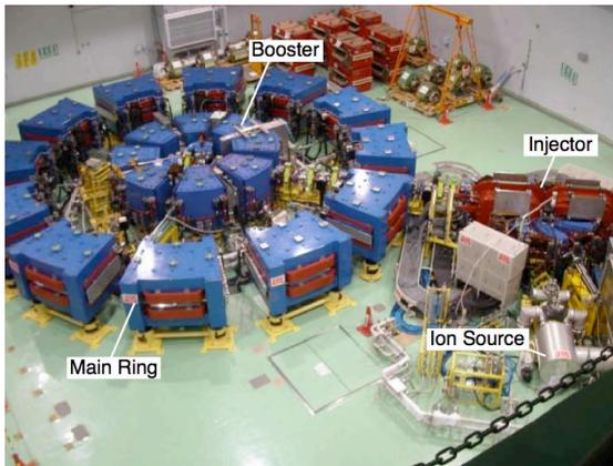
ADSR FFAG (present): Combined with a reactor, it demonstrates Accelerator Driven System.
