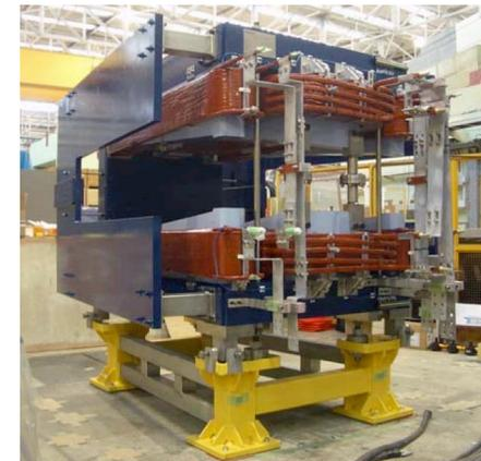
PRISM FFAG (present): Muon phase rotator to reduce momentum spread.
