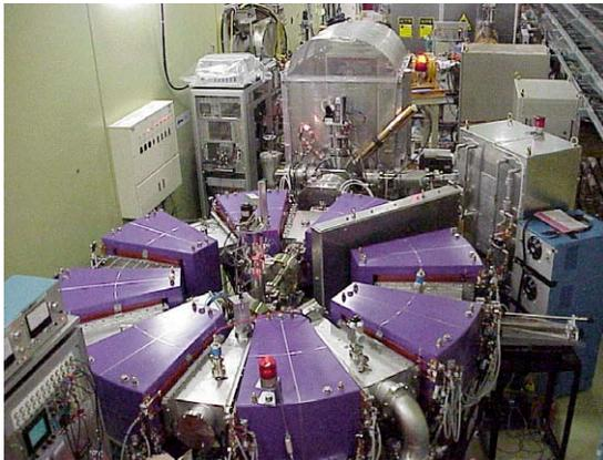
PoP FFAG (2000): The world's first proton FFAG with MA rf cavity.
