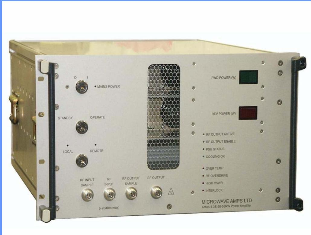
650 W, 1.3 GHz driver developed for XFEL
