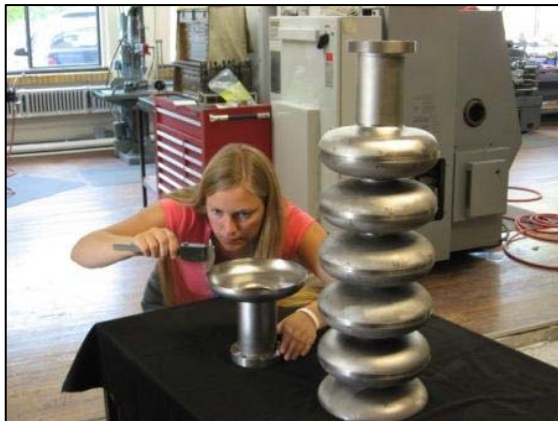
1.3 GHz \beta=0.81 seven-cell cavities
