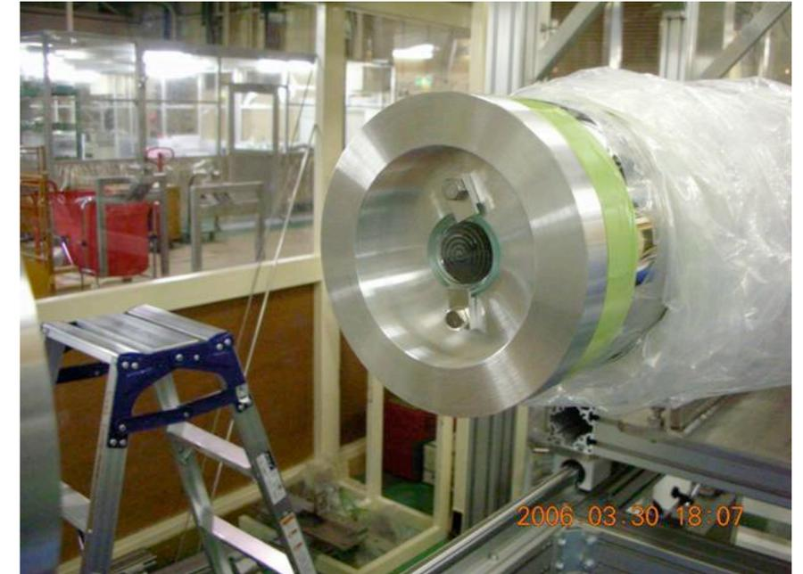
Decide the axis of the coaxial coupler set in the cryostat by using transit.
