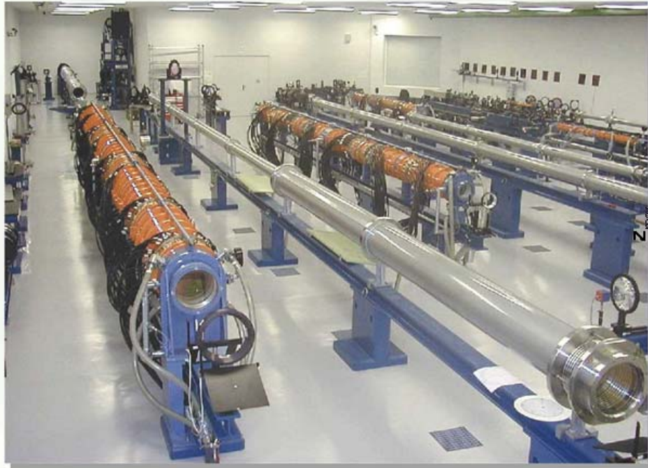
Iodine laser at the PALS Research Center in Prague \lambda = 1.315 \mu\text{m} , E \leq 1 \text{ KJ} , 8 \times 10^{16} \text{ W/cm}^2
