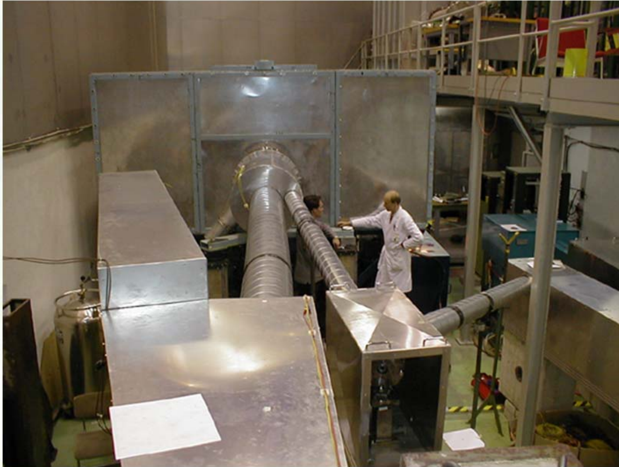
100 J/1 Hz MO-PA CO 2 -laser system
