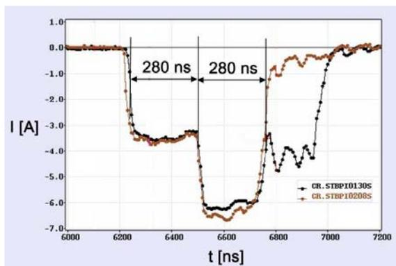
Figure 6: First recombination in the Combiner Ring. The traces show the beam current in 2 BPMs. The incoming beam pulse has twice the length of the ring (2 x 280 ns). During the second part, the bunches are interleaved with the bunches that made one revolution in the ring.
