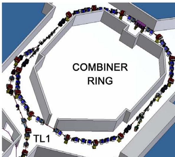
Figure 2: Combiner ring layout. On the left the transfer line from the delay loop to the ring is also represented.
