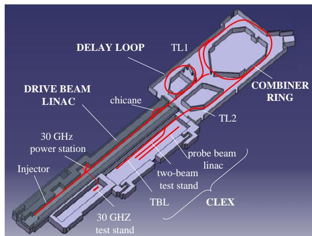
Figure 1: Schematic layout of the CTF3 complex.
