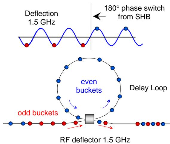
Figure 3: Schematic of the delay loop recombination.
