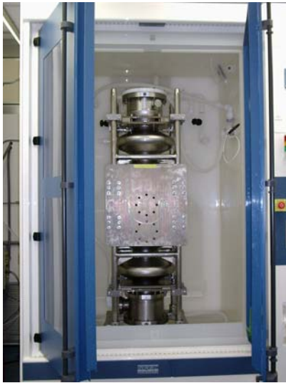
Figure 2. The closed chemistry, BCP, cabinet is used to acid etch the inner surface of the cavity at a controlled etch rate and temperature.
