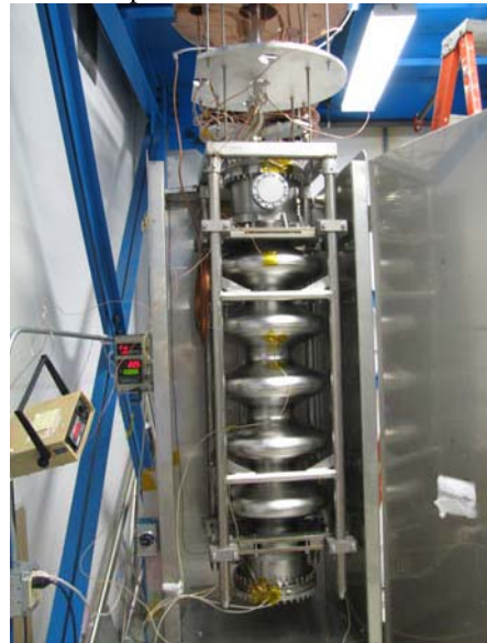
Figure 4. The low temperature bake-out box used for the 5 cell cavity 110 degree bake.
