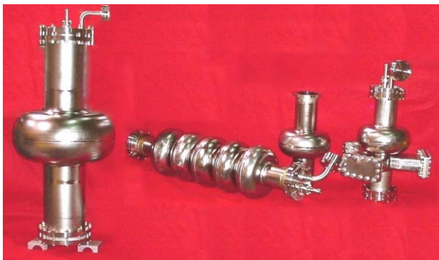
Figure 3: 748.5 MHz and 1497 MHz High-current prototype cavities.
