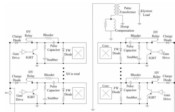
Figure 1: Schematic of solid state modulator.
