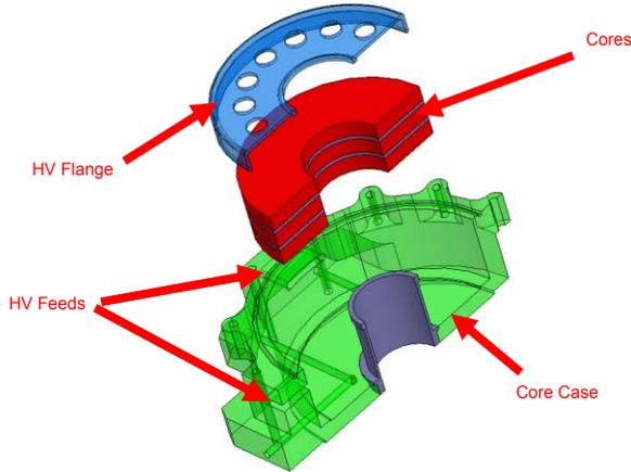
Figure 2: Core case assembly.
