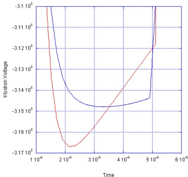
Figure 5. SPICE results of RL compensated (blue), and uncompensated (red) pulses.
