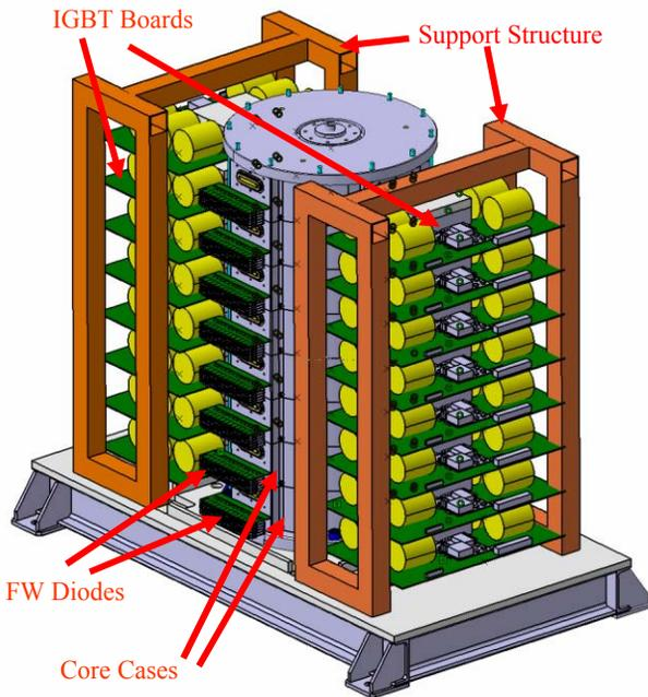
Figure 3: Assembled solid state modulator.
