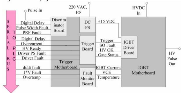
Figure 4. Block diagram of cell electronics.
