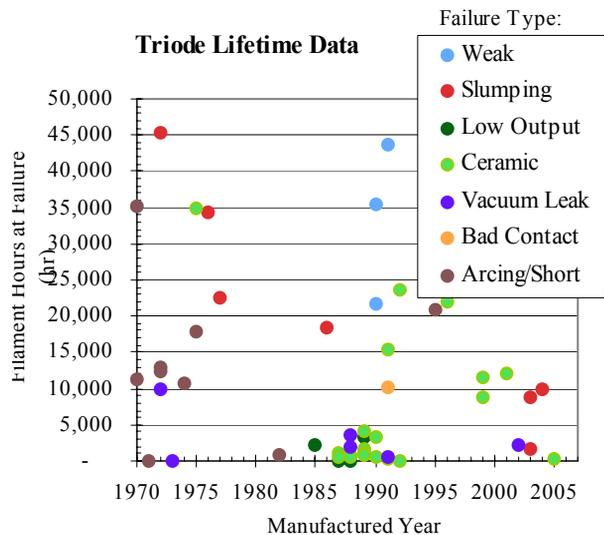
Figure 3: Summary of Triode Failures.
