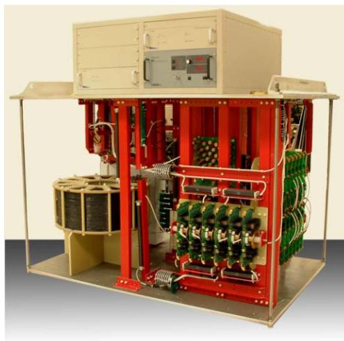
Figure 1: Photograph of the modulator. To the left is the bouncer inductor; the bouncer capacitor can be barely seen behind it. The six circuit boards in the lower right are the bouncer switches. At the far right are the main switches. The bouncer supply is mounted in the rack on top, where the control electronics will also be installed.
