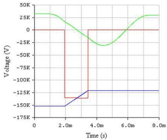
Figure 5: Voltages in the ILC hard switch. Top trace, voltage on the bouncer capacitor; bottom trace, voltage on the main capacitor; middle, combined output voltage. The bouncer circuit compensates for 31 kV of droop during the pulse.
