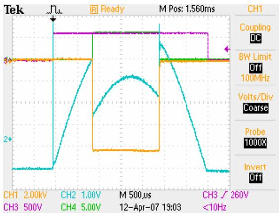
Figure 7: Test showing that the capacitor droop is compensated over the full 1.5-ms pulse. Channel 1 is the output voltage, 4 kV/div. Ch 2 is the current in bouncer capacitor, 10 A/div. Chs 3 and 4 are pulse commands.
