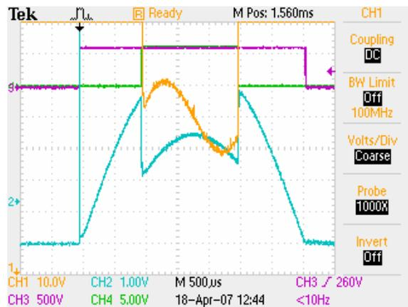
Figure 8: Test at higher sensitivity. Ch 1 is the output voltage, at 20 V/div. The ripple is  $\pm 24$  V out of 16 kV, 0.15% for the conditions here.
