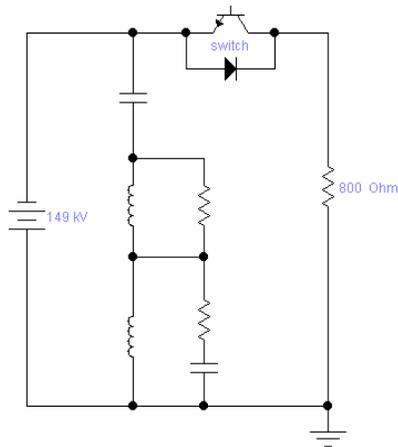
Figure 4: Passive bouncer circuit. The up LR section provides the main droop correction; the lower LRC section reduces the initial voltage spike. The stored energy and power dissipation are too large for this to be practical for ILC.
