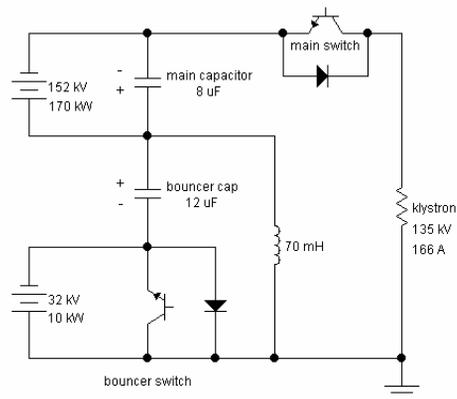
Figure 2: Simplified schematic of the hard-switch modulator. The inductor is sized such that the pulse length is about one quarter of the bouncer period.
