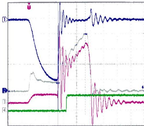
Figure 3: Opening switch arc response. Trace 1 shows cathode voltage, with the arc occurring at full voltage. Traces 2 and 3 show switch and cathode current, respectively. Trace 4 is the internal switch control. Detection of the arc, and the command for the switch to open requires  $\sim 200$  ns from arc onset, with full switch opening in  $\sim 600$  ns, as shown by the falling currents.
