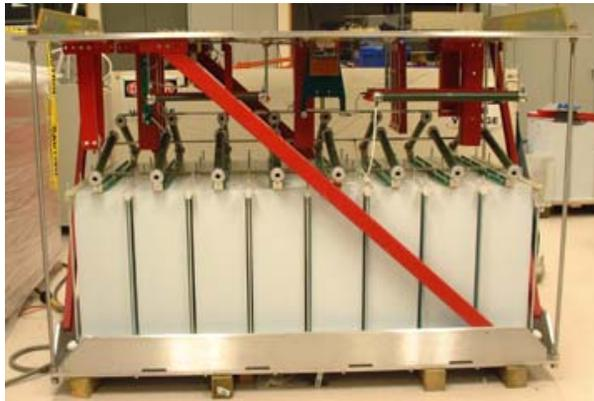
Figure 6: Capacitor bank for the ILC hard-switch modulator. The bank has a capacitance of 8  $\mu$ F, a voltage of 150 kV, and stores 90 kJ.
