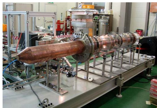
Figure 4. 700 MHz PEFP prototype klystron tube after the final welding
