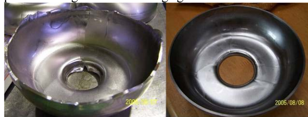
Figure 2: Half-cell after deep-drawing and trimming.
