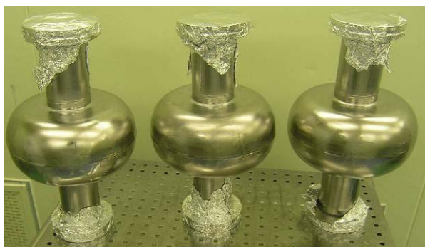
Figure 1: Three 1.3 GHz cavities by using China large grain niobium.
