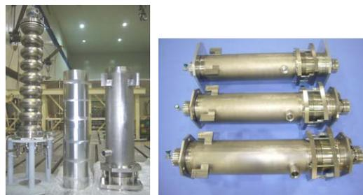
Figure 9: Before and after welding of a He jacket. A magnetic shield (centre in left) was inserted in a He jacket.
