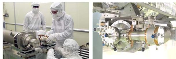
Figure 10: Installation of an input coupler (Left) and an assembled cavity mounted on 2 K gas return pipe (Right).
