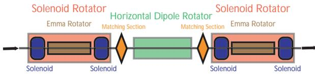
Figure 1: The ILC Spin Rotator schematic.
