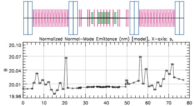
Figure 2: Vertical normalized emittance growth in the Spin Rotator (in nm).
