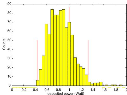
Figure 7: Empirical bootstrap distribution for the return level with a probability of 0.99. The two small red marks indicate the  $\pm 2\sigma$  interval, the big red mark indicates the return level obtained with a direct estimate from the recorded losses.
