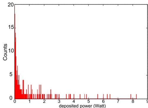
Figure 3: Unnormalized probability density function for the losses at the first quadrupole of the first section. The deposited beam power (W) forms the abscissa and the number of counts the ordinate.
