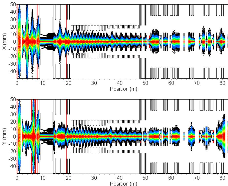
Figure 1: The deuteron density projection in the transverse plane in the SPIRAL2 linac (the black line is the aperture).
