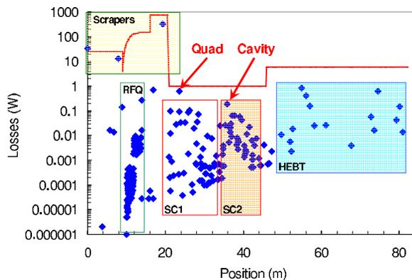
Figure 2: Average loss repartition along the structure. The most critical components are pointed with red arrows.
