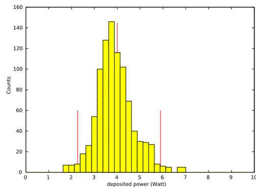
Figure 5: Empirical bootstrap distribution for the return level with a probability of 0.97. The two small red marks indicate the  $\pm 2\sigma$  interval, the big red mark indicates the return level obtained with a direct estimate from the recorded losses.
