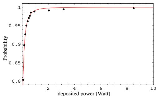
Figure 6: GEV fitted with the recorded losses for the most critical cavity. The deposited beam power (W) forms the abscissa and the CDF the ordinate.
