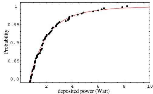
Figure 4: GEV fitted with the recorded losses for the quadrupole. The deposited beam power (W) forms the abscissa and the CDF the ordinate.
