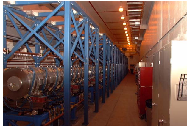
Figure 3. The DARHT 1 st axis accelerator consists of a 3 MV injector and 64 induction cells, each cell operating at 250 kV to produce a 19 MeV, 1.9 kA, 60 ns electron beam. The electron beam is focused onto a Tantalum target, generating a 625 Rad X-ray pulse having a spot size diameter of less than 2.0 mm (MTF).
