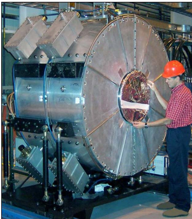
Figure 5: All accelerator cells have been refurbished and tested at LANL.
