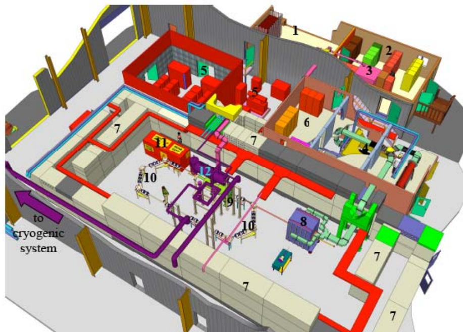
Figure 1: Layout of R&D ERL in Bldg. 912 at Collider-Accelerator Department, BNL: 1 – R&D ERL control room; 2 – diagnostic and control racks; 3 – 703.75 MHz, 50 kW CW RF transmitter; 4 - 703.75 MHz, 1 MW CW klystron; 5- 2 MW CW HV power supply for the klystron; 6 – power supplies and other electronics; 7 – shielded R&D ERL vault with removed roof beams; 8 – 2 MeV, 703.75 MHz SRF photo-injector; 9 – 20 MeV, 703.75 MHz 5-cell SRF linac; 10 – return loop; 11 – beam dump; 12- part of the 1.8 K o cryogenic system (most of the system is outside the picture).
